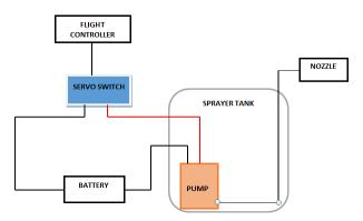
Fig. 3.2 Block diagram of spraying system
