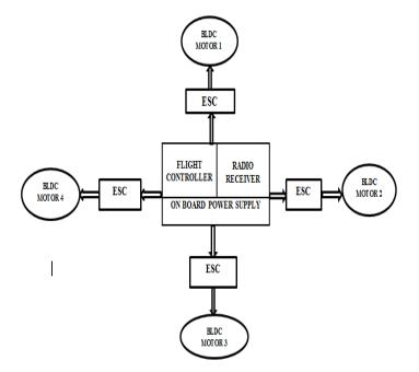
Fig. 3.1 Block diagram of Quad copter
